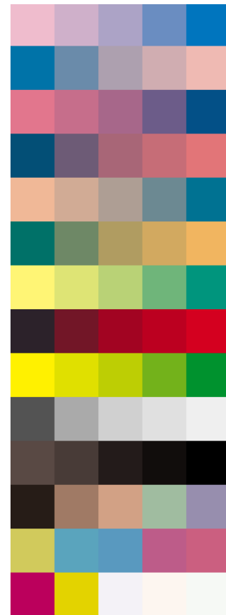
This segment of a test target shows rows of color patches measured by a spectrophotometer to make a ColorSync profile. Using the profile, ColorSync can be instructed to make a color-correct separation that takes all qualities of the device into account.
